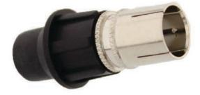
Product code: KFMQ Connector: Quick F male (61169-24) Material: brass Finish: nickel Type: straight Unit weight: 7,0 g Package: 100 pcs Certifications: CE – RoHS – SCTE
