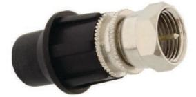
Product code: KFM Connector: F male screw-on (61169-24) Material: brass Finish: nickel Type: straight Unit weight: 7,5 g Package: 100 pcs Certifications: CE – RoHS – SCTE
