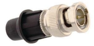
Product code: KBM Connector: BNC male (61169-8) Material: brass Finish: nickel Type: straight Unit weight: 11,9 g Package: 100 pcs Certifications: CE – RoHS – SCTE
