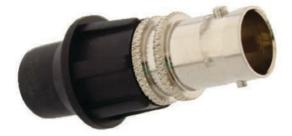
Product code: KBF Connector: BNC female (61169-8) Material: brass Finish: nickel Type: straight Unit weight: 7,4 g Package: 100 pcs Certifications: CE – RoHS – SCTE
