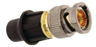
Product code: KBM-HQ Connector: BNC male (61169-8) Material: brass Finish: gold and black nickel Type: straight Unit weight: 9,5 g Package: 100 pcs Certifications: CE – RoHS – SCTE
