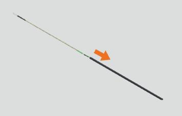
4. Pulling from the two flaps, strip the pre-engraved sheath for the necessary length in order to easily manage the fiber and cut the excess of the sheath and the Kevlar
