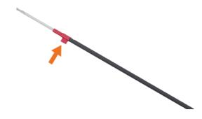
3. Gently slide the sheath along the fiber by gripping the top of the sheath
