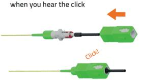
Easy Fiber 11. Remove the ferula temporary protection and insert the green cap
